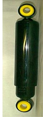
Because shocks deteriorate over time, most people don't notice the changes. It stands to reason then that shocks are an item that should be regularly inspected. Many people do not realize that driving with worn shocks is as risky as using brakes well past their prime or driving on bald tires. It is extremely dangerous when needing to maneuver in emergency situations.
